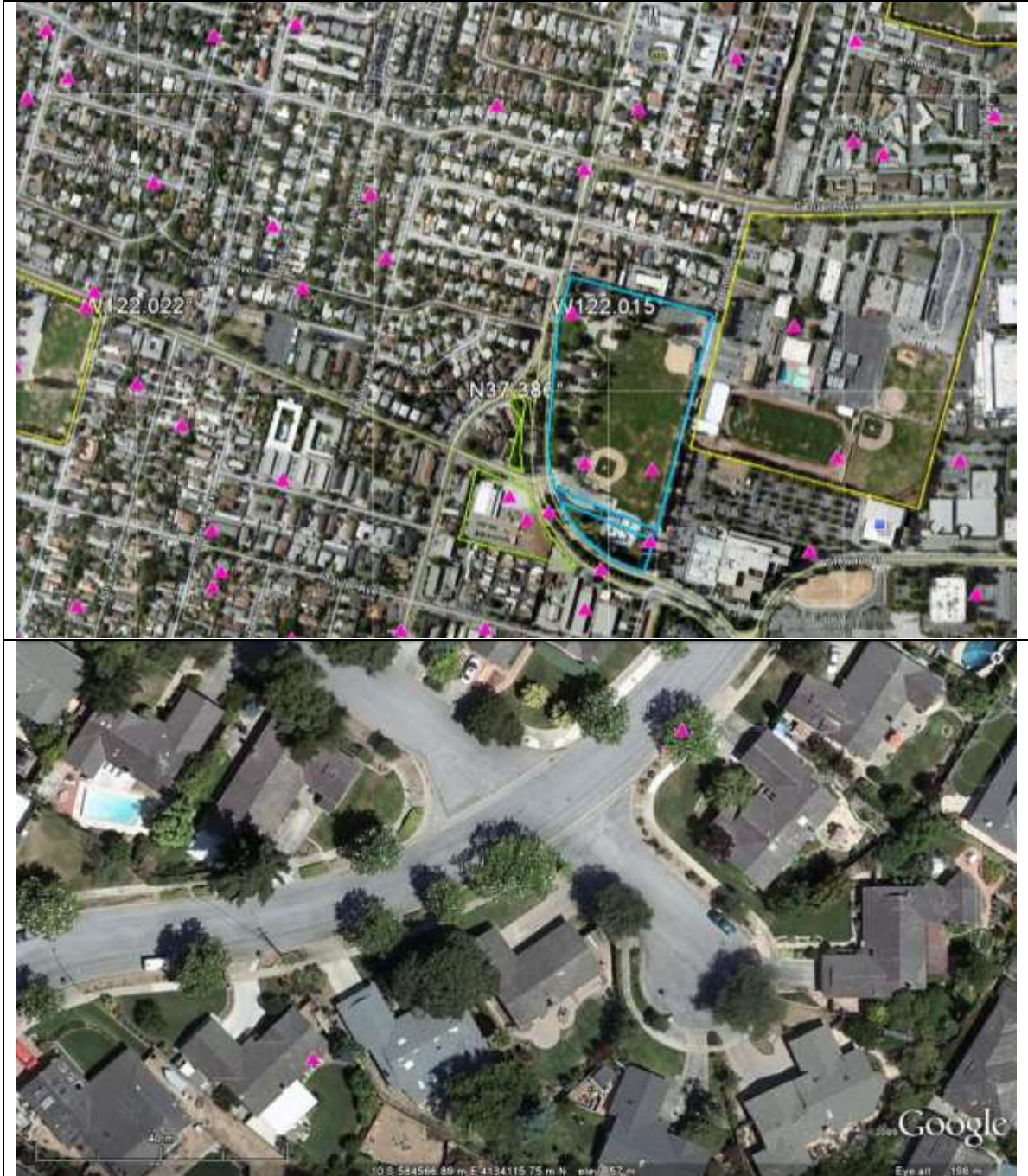
Figure 3-5. Aerial imagery of Sunnyvale (photo date July 2007) used for determining tree canopy cover. Top image shows the distribution of random points across a section of the city with polygon boundaries that indicate specific land uses (blue line = a city park, yellow line = school, green line = other city owned property). Latitude/longitude grids were used to help keep track of position during the counting process. Determination of whether sample points intercepted tree canopy were made under greater magnification, as shown in bottom image. Lower image shows a close-up with two sample points, one on a street tree (upper right) and the other on non-canopy beyond the ROW (lower left) within a residential area. The apex of each triangle was used as the actual sampling point. Imagery: Google Earth.
